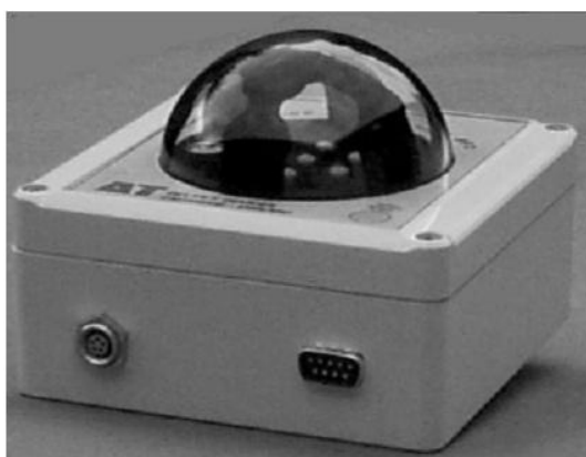
Figure 1: The BF2 Sunshine Sensor, Source: Sunshine Sensor Type BF2 User Manual, Delta-T Instruments, Burwell, Cambridge, Version 1b, 25 th March 1999.
